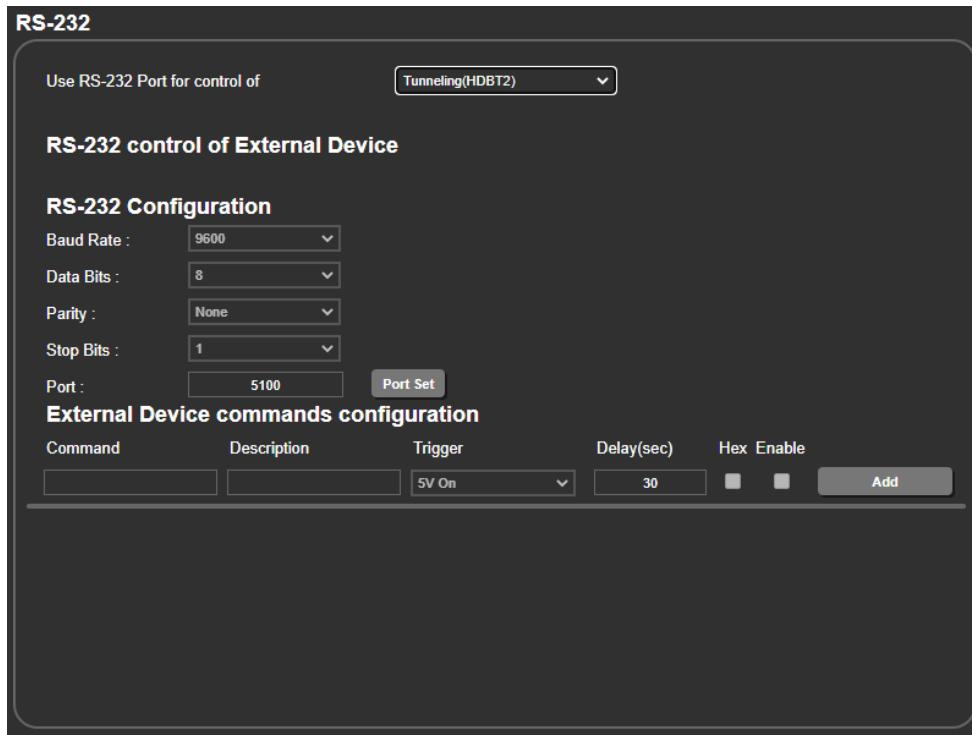
Figure 37: RS-232 Page – Controlling an External Device via HDBT Tunneling
