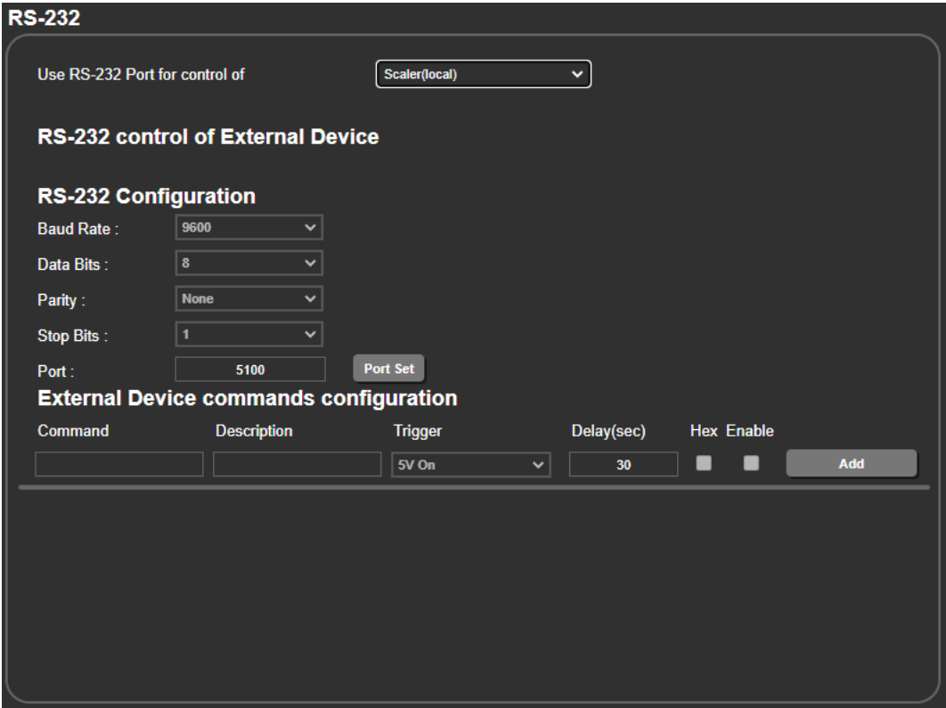
Figure 28: RS-232 Page – Controlling the VP-427X2
